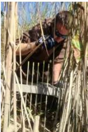
Surface Elevation Tables
